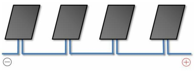
A solar array made of four solar panels connected in series. If each individual panel is rated as a 12-volt, 12-watt panel, this solar array would be rated as a 48-volt, 48-watt array with a 1 amp current.
