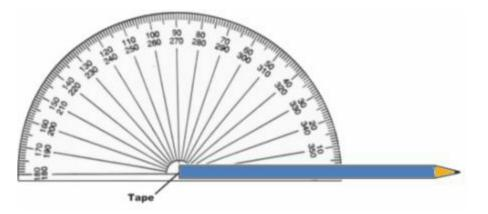
Tape the pencil to the centre of the protractor where all the lines meet, in such a way that the other end of the pencil can be moved across the protractor. You can use this protractor to check the field of view, using the pencil as an 'aimer' to measure the angle of nearby obstacles relative to your location.
