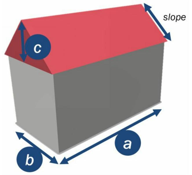
You will need to measure and record the overall roof-space available for your solar array. There are various ways of doing this, but the easiest way is to measure the footprint of the building at ground floor level, measure the height of the roof from within the attic space and then calculate the size of the roof from this.
