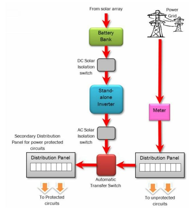
In this above diagram, a second consumer box has been wired into the electrical system, with power feeds from both the main consumer box and an inverter connected to a solar system.
