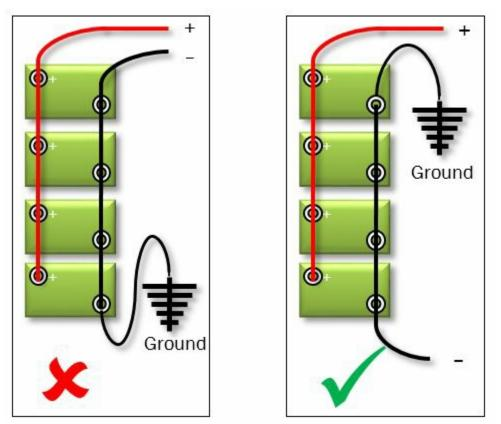
How to wire batteries in parallel: the diagram on the left, where power feed for both positive and negative is taken off the first battery in the bank, shows how **not** to do it – it will lead to poor battery performance and premature battery failure. The diagram on the right, where the positive feed is taken off the first
