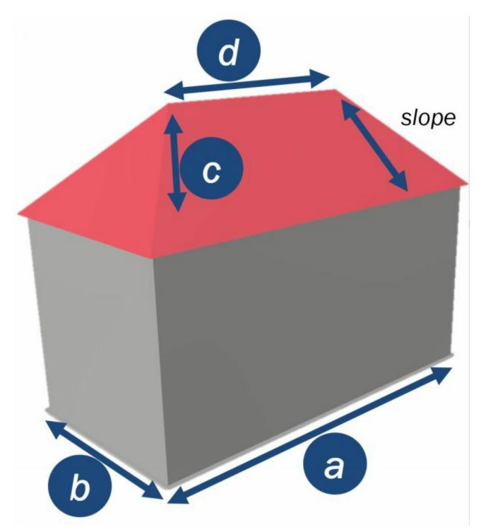
If you have a hip roof, like the one shown above, your calculation will be a little more complicated. A hip roof is a type of roof where all the sides slope downwards to the walls. An absolutely accurate calculation to work out precisely the amount of space available with a hipped roof can get very convoluted. However, there is a quick and simple ready-reckoner calculation that is accurate enough unless you are trying to squeeze every last solar panel onto the roof.
