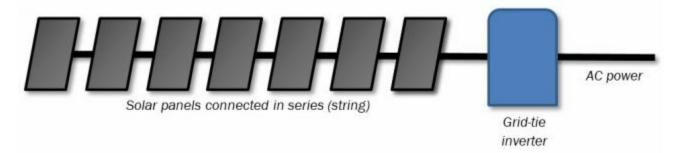
A simplified block diagram showing the basic layout of a high voltage in-series solar energy system
