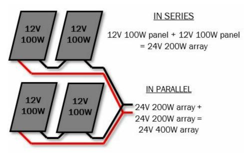
A sample diagram of a 24-volt array where two sets of two 12-volt
