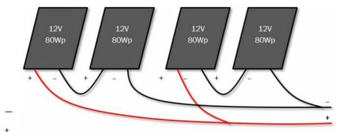
This drawing shows how I intend to wire up my solar array. I will pair two sets of panels together in series to bring the voltage up from 12 volts per panel to 24 volts per pair. I then connect the pairs together in parallel to maintain the 24 volts but to increase the power of the system to a total of 320 watts
