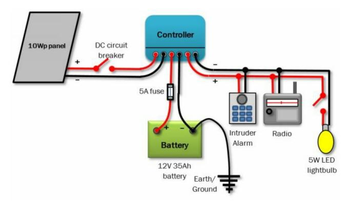
Above: A simple solar installation: a light with light switch, a small radio and a simple intruder alarm – perfect for a beach hut, garden shed or a small lock-up garage. Because it is a small system, you may choose not to fit an isolation switch. Because the system is very small, I have decided only to fit a fuse between the controller and the battery
