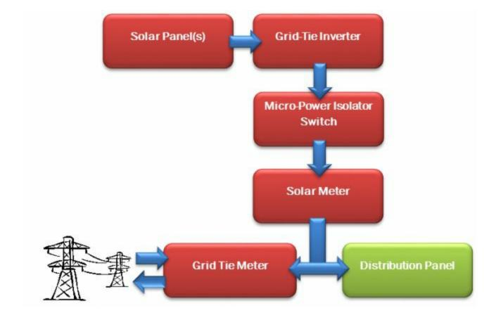
This simplified block diagram shows a simple grid-tie system, typical of the type installed in many homes today. The solar panels are connected to the grid-tie inverter, which feeds the energy into the main supply. Electricity can be used by devices in the building or fed back out onto the grid, depending on demand.
