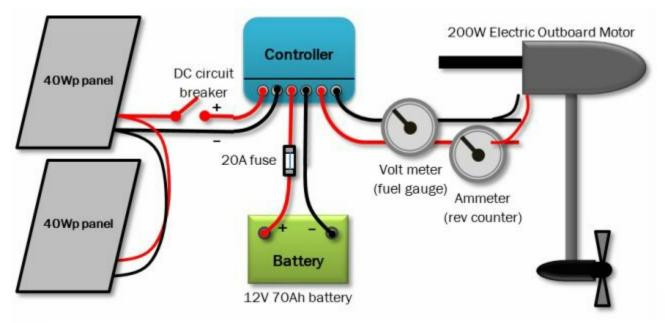
Above: A solar powered river boat. Electric boats are terrific on the river; the only downside is recharging the batteries. Here, solar panels are used to recharge the batteries, charging them up during the week to provide all the power required for a weekend messing about on the river.
