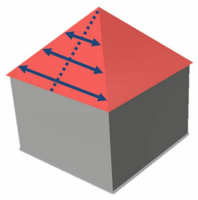
Measure 120cm (48 inches) down from the top of the roof along the pitch of the roof, and measure the width of the roof at this point. Deduct 60cm (24 inches) from this measurement to take into account that you cannot fit solar panels too close to the edge of the roof.
