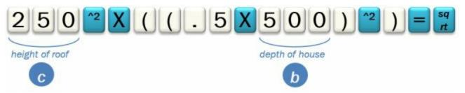
In this example, the answer is 353.5cm. This means the slope of your roof (measurement d in the diagram at the top of the page) is 353.5cm (139 inches).
