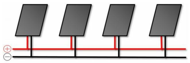
A solar array made of four solar panels connected in parallel. With each panel rated as a 12-volt, 12-watt panel, this solar array would be rated as a 12-volt, 48-watt array with a 4 amp current.
