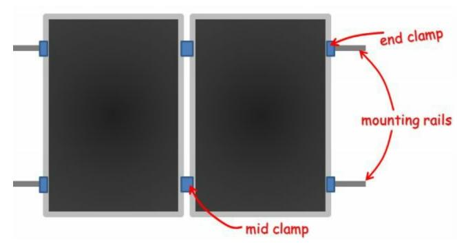
Self-locking nuts should be used to ensure the panels remain firmly clamped. Solar panels suffer from wind buffeting over time, which can loosen bolts. Some frame clamps are designed to vibrate tighter with buffeting, reducing the risk of panel damage over time.
