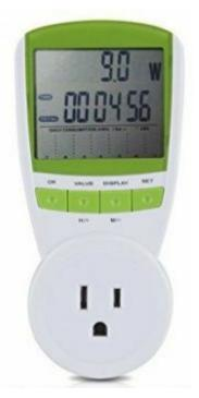
A watt meter, like the example shown above, is a useful tool for measuring the energy requirements of any device that runs on high-voltage AC power from the grid. The watt meter plugs into the wall socket and the appliance plugs into the watt meter. An LCD display on the watt meter then displays the amount of power the device is using. This is the most accurate way of measuring your true power consumption.
