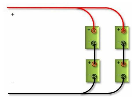
This drawing shows how I intend to wire up my batteries. I will pair two sets of batteries together in series to bring the voltage up to 24 volts per pair. I then connect the pairs together in parallel to maintain the 24 volts but to increase my storage capacity to 210 amp-hours at 24 volts
