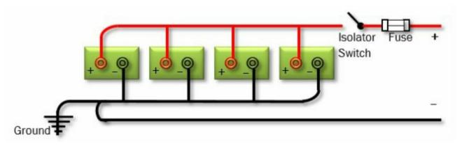
Four 100-amp-hour 12V batteries connected in parallel to provide a 400-amp-hour 12V battery bank.
