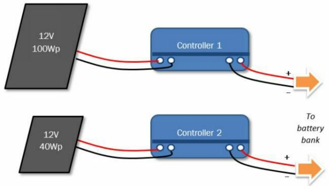
This system uses two controllers. The second controller is used to provide additional power to the batteries for the smaller solar panel. Both controllers charge the same battery bank.
